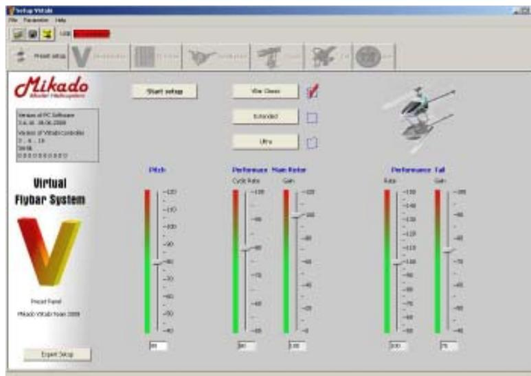
Using the control bar for the main and tail rotor you can adjust the flight properties of the helicopter.
