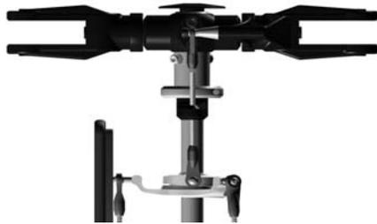
3) It is necessary to install a swashplate driver. Mikado offers a swashplate driver for 10 mm main rotor shafts. It has eight ball bearings:
